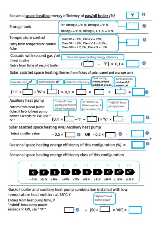
Figure 2: elements of the fiche for cogeneration boilers as related to the seasonal space heating energy efficiency of their combinations with further products
