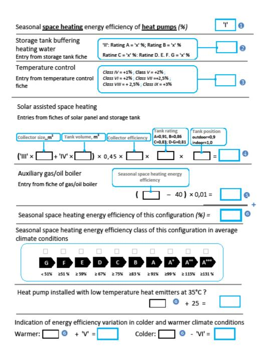
Figure 4: elements of the fiche for low-temperature heat pumps as related to the seasonal space heating energy efficiency of their combinations with further products
