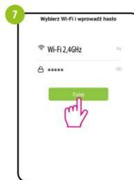
Select the Wi-Fi network in which the thermostat will operate and enter the password of this network.
