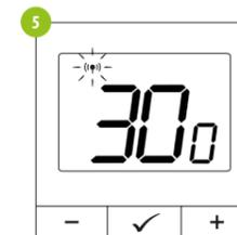
The thermostat started to send a signal (☉) to find the receiver and started the countdown with the number 300 (sec). The pairing process may take up to 300 seconds.
