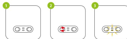
If you want to re-pair the receiver and thermostat with each other and then add it to the application, make sure that the receiver is disconnected from the power supply, and the switches on it are in the ON and AUTO positions. Then connect the receiver to the power supply and wait a few seconds. Next, move the left switch to the OFF position and back to the ON position with a quick motion. The orange LED will start blinking, which will confirm that the receiver has entered the pairing mode.
