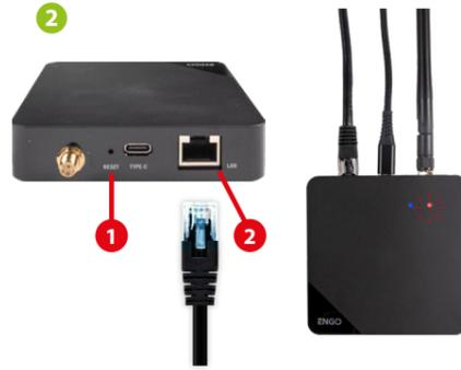
Make sure the device is connected to the power supply and to the Internet via the cable (2). Then press and hold the RESET button (1) (using the pin provided) for 10 seconds. The red LED must flash slowly, then the gateway is in pairing mode. If the red LED flashes quickly, then press the RESET button again for 10 seconds, wait a moment and make sure that the red LED flashes slowly.
