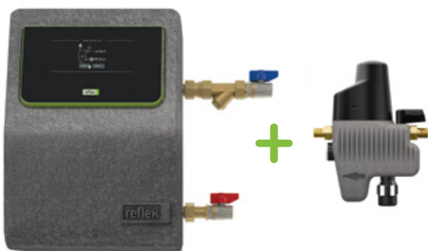
Automatic make-up takes place independently via the Fillcontrol Plus Compact
