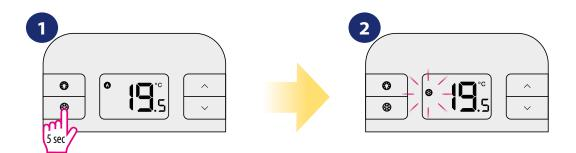
By default thermostat is in HEATING mode (flame icon is displaying). To change the thermostat into the COOLING mode — press and hold the SNOWFLAKE button for 5 seconds.
