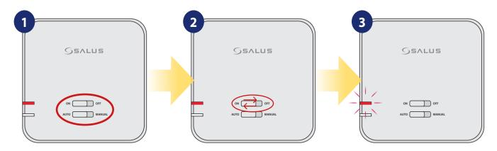
If you want to re-pair the devices with each other, make sure that the receiver is disconnected from the power supply and the switches on it are in the AUTO and ON positions. Then connect the receiver to the power supply and wait for the red diode to glow continuously.
