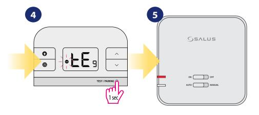
Press TEST / PAIRING button again to return to the main screen.
