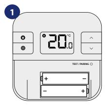
Remove the batteries without pressing any button. Wait 2 minutes and insert the batteries again. Your device will be restarted.
