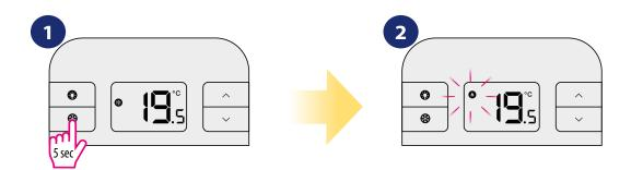
To change the thermostat into the HEATING mode — press and hold the SNOWFLAKE button for 5 seconds.
