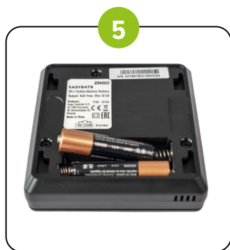
5 Insert batteries in the thermostat
