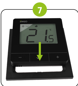
7 Attachment of regulator to mounting plate The thermostat in the frame is ready for operation
